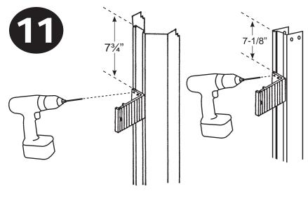
Before assembling your pool, drill the required holes in the Verticals and Buttress post.
